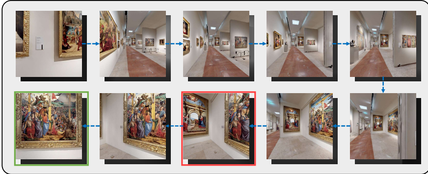
Figure 8.4: An episode of PointNav++ in AG3D where consecutive frames have a distance of 10 timesteps approximately. The red frame indicates the stop action in the traditional PointNav task. The green frame corresponds to the stop action in PointNav++.
